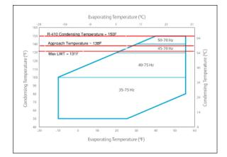
The *approach* is determined by the plate heat exchanger sizing, which must maximize heat transfer and ensure oil return to the compressors. For R-410a machines, the *approach* is typically 10.8F - 12.6F degrees.
