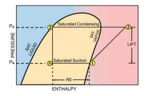
The image to the right is a typical pressure-enthalpy (P-H) diagram for refrigerant. Everything to the left in blue is 100% liquid and everything to the right in red is 100% vapor. The yellow region is a mixture of liquid and vapor.
