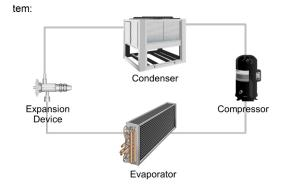
**Condenser:** This is where high pressure refrigerant gas condenses back into a highpressure liquid. The heat required to condense the refrigerant typically comes from air or water which in turn is exhausted into the ambient air.
